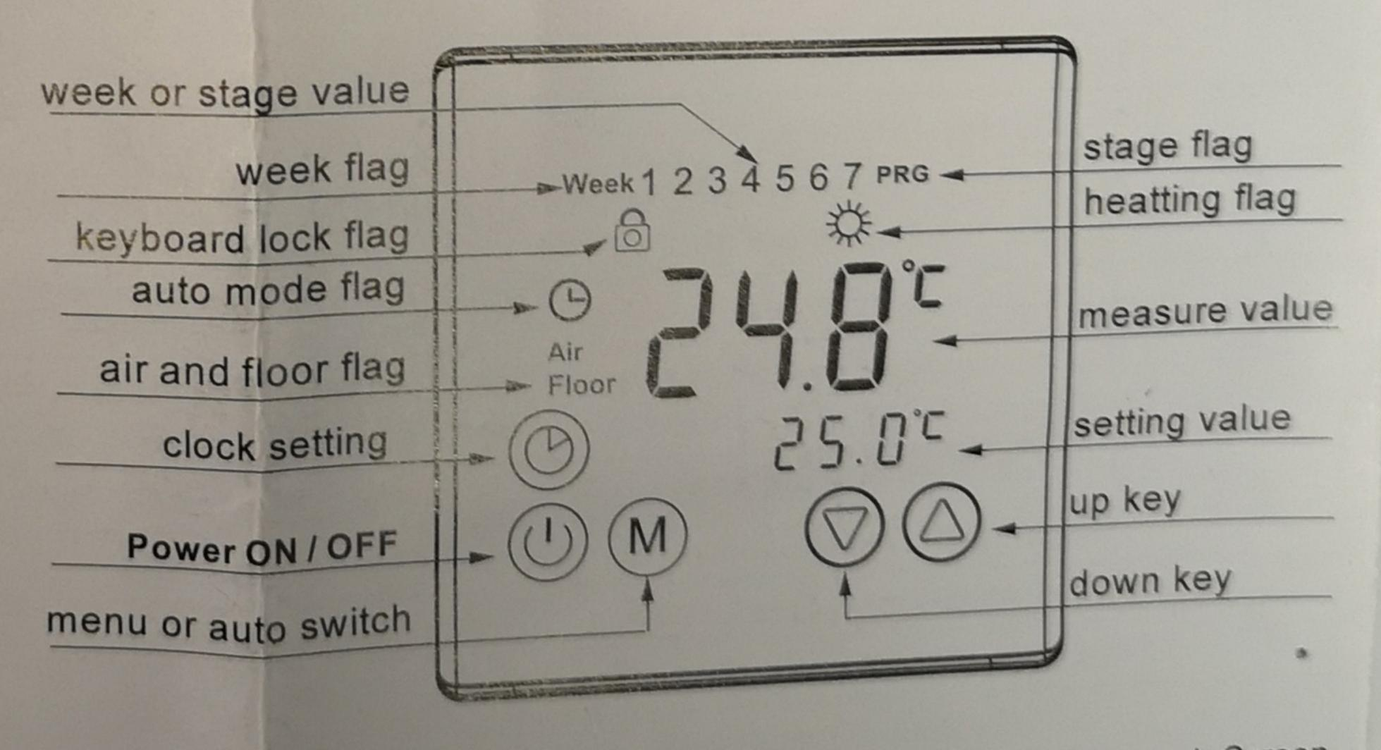
[ Children Lock ] Press key ( M) for 2 seconds at the same time, the controller keypad would be locked. Screen would show . Press the ( M) at the same time for 2 seconds under the locked status, keypad would be unlocked.
